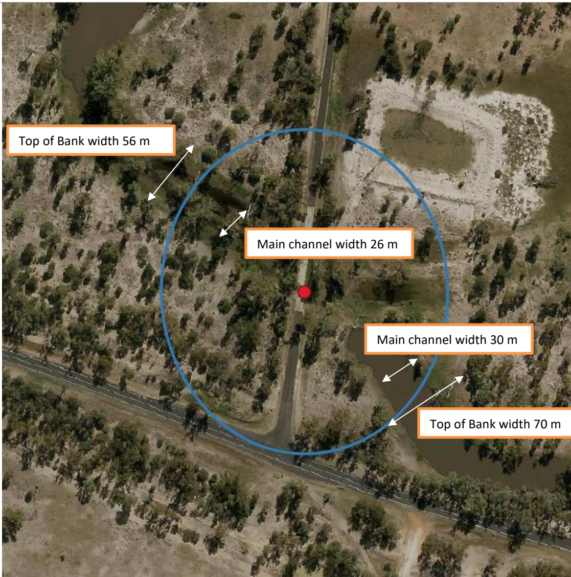
Creek measurements upstream and downstream from crossing
